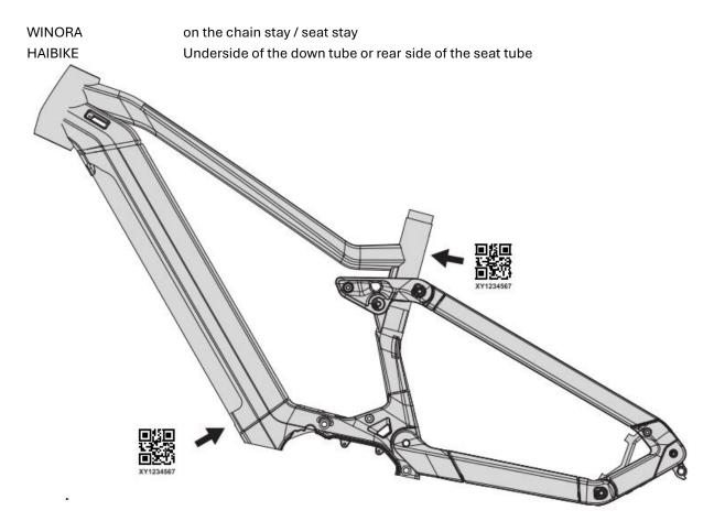
GHOST, LAPIERRE: Down tube by the fork or in the bottom bracket / motor area
